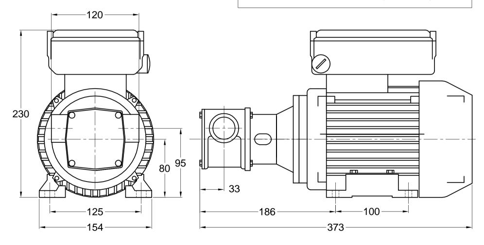
MOTOR DIMENSIONS MAY VARY ACCORDING TO MAKE AND TYPE FITTED dimensions in mm
